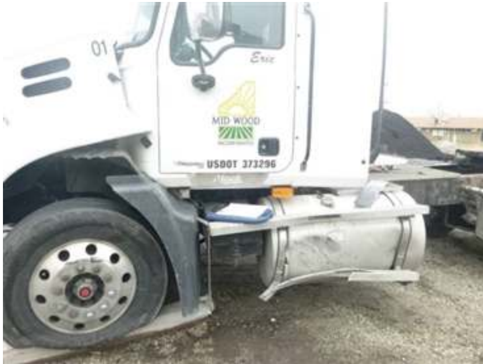
Document Name: P1050460.JPG Remarks: Lt fuel tank and step damage
