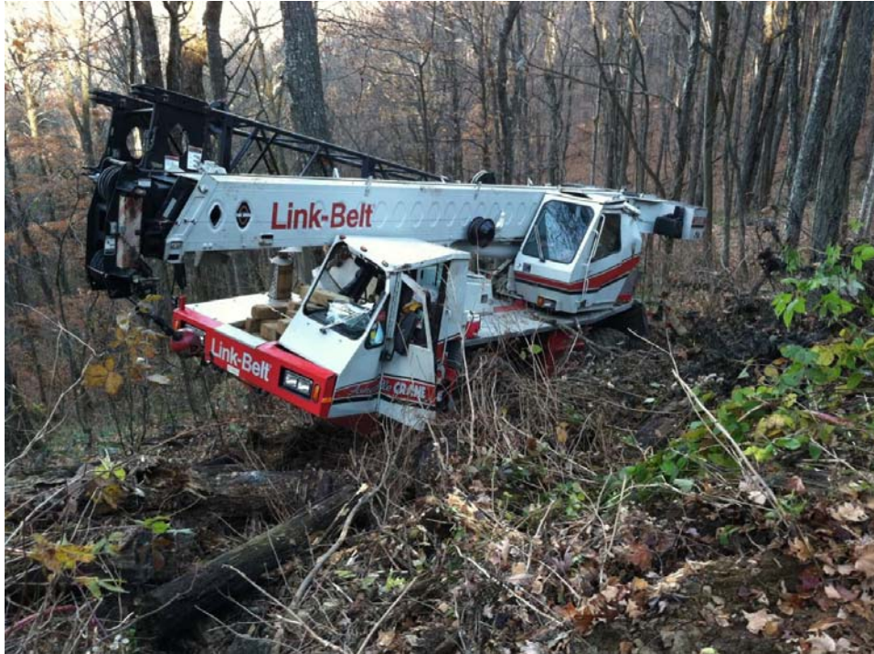
Photo #1: View of 2003 Linkbelt ATC-822, 22-ton, All-Terrain Crane SN: 71J35776, with 70' main and 45' jib.
