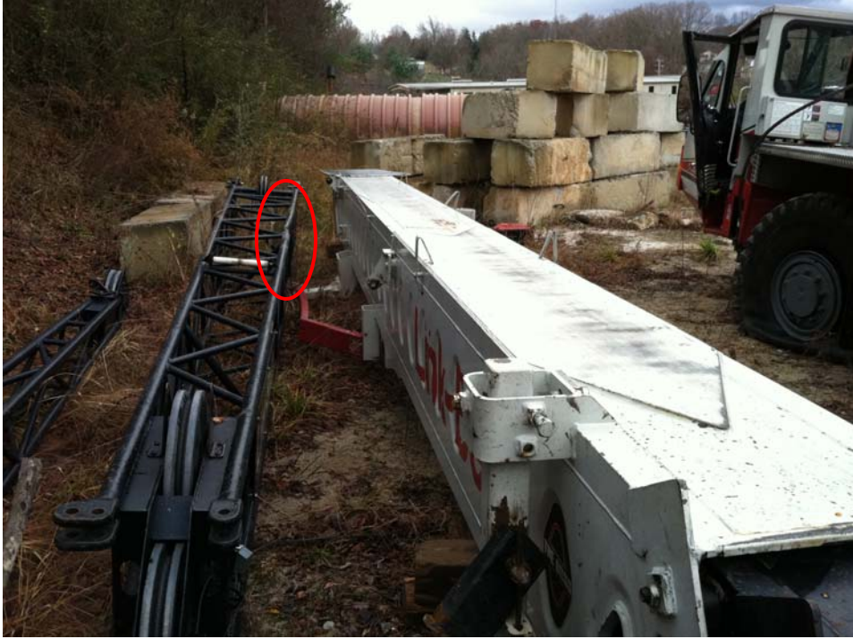
Photo #15: View depicting boom and jib. Damage to jib from impact. No visible damage to boom.
