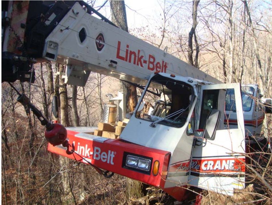
Photo #5: Front view – depicting damage to carrier cab.
