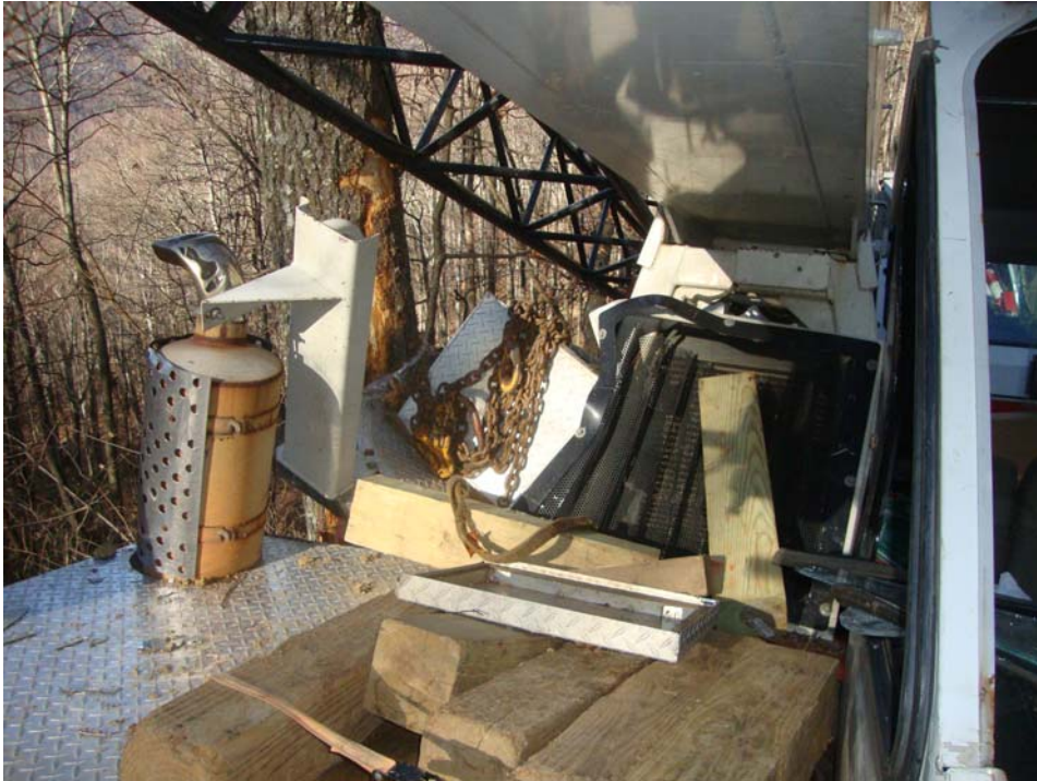
Photo #19: Radiator/Cooling system sustained damaged from impact.
