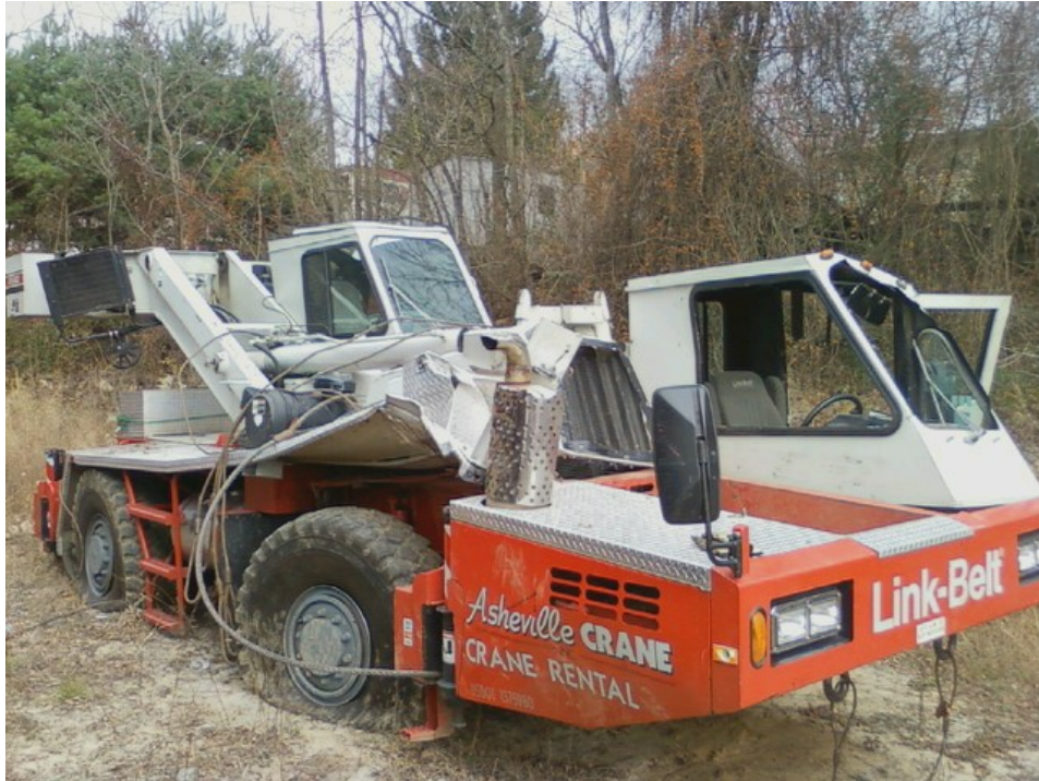
Photo #13: Right side view of boom truck recovered from site. Boom has been removed.
