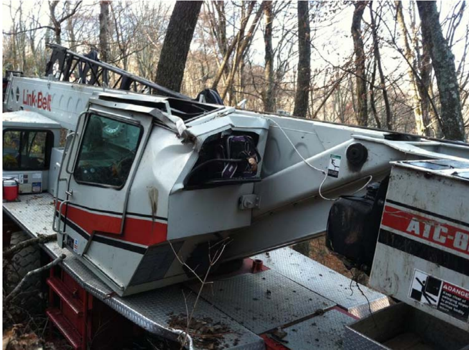
Photo #3: View depicting damage to boom cab and aluminum decking.
