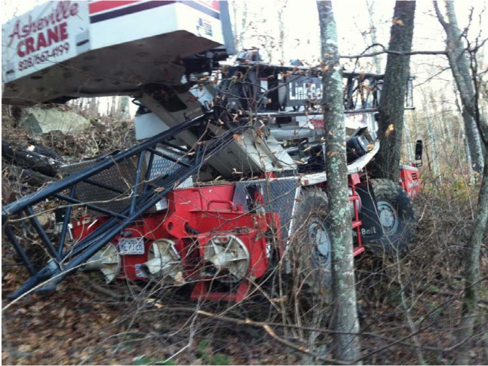
Photo #7: View depicting damage to jib and fly.
